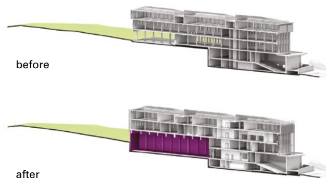
Underspinning the Tapestry Nave : how to optimize the building structure and create an exhibition space with monumental dimensions.
